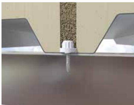
Opticore is EJOT's unique and patented integral nylon head, designed to encapsulate fasteners from our high performance Self-Drilling range. Opticore is engineered to provide a dual drive fastening system that enables rapid self-coring of membrane faced insulation panels, and a secure fix into hot and cold rolled steel, and timber.
