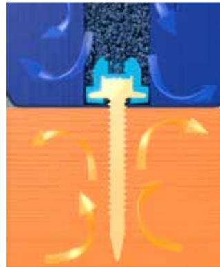
Hot box tests and thermal activity recording has repeatedly shown that the composition of the Opticore head provides better thermal retention values over metal fasteners.
