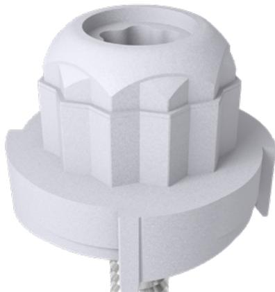
The intergral Opticore head design is manufactured in high strength moulded nylon. The 'cutting fins' are unique to the Opticore patent, and create the smooth coring of the panel's insulation. On secure 'pull-up' of the fastener into the substrate, the fins simply snap away without any compromise to the integral lining.
