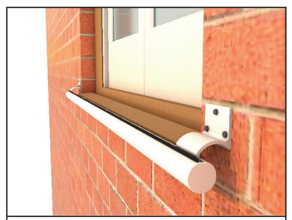
3. When properly lined up fix the bottom track brackets firmly to the wall. (use a level to make sure you are horizontally level)
