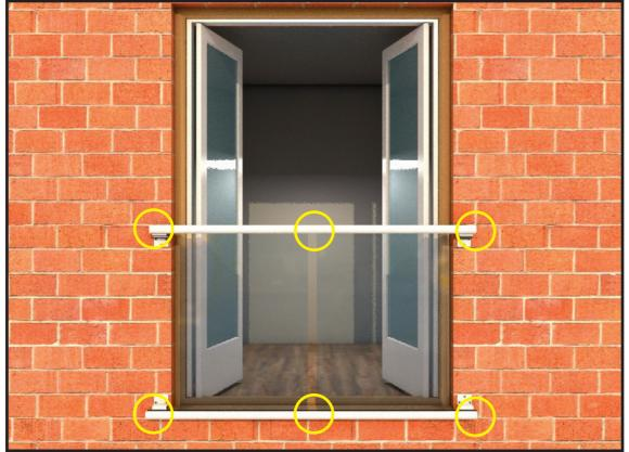
12. Line the glasses up in position so that they are spaced correctly between each other/wall etc.
