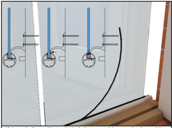
13. Insert the 3mm rubber gasket in the bottom track between the glass and the glazing bead. (using soap water can ease the process)
