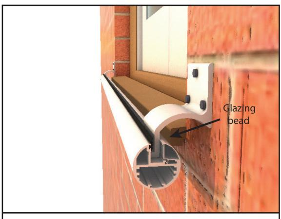
2 . Line up bottom track vertically to allow the access to the glazing bead from the inside.
