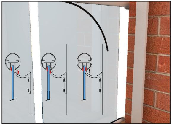
14. Insert the two 3mm rubber gaskets on both sides of the handrail. (using soap water can ease the process)
