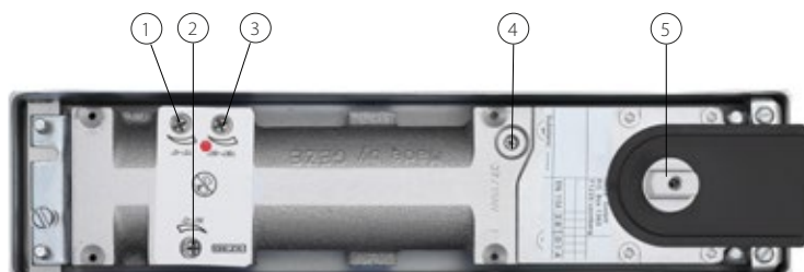
1 = Latching action setting | 2 = Closing speed setting | 3 = Hold-open function setting / closing delay | 4 = Closing force setting | 5 = Frontal gearing pivot
