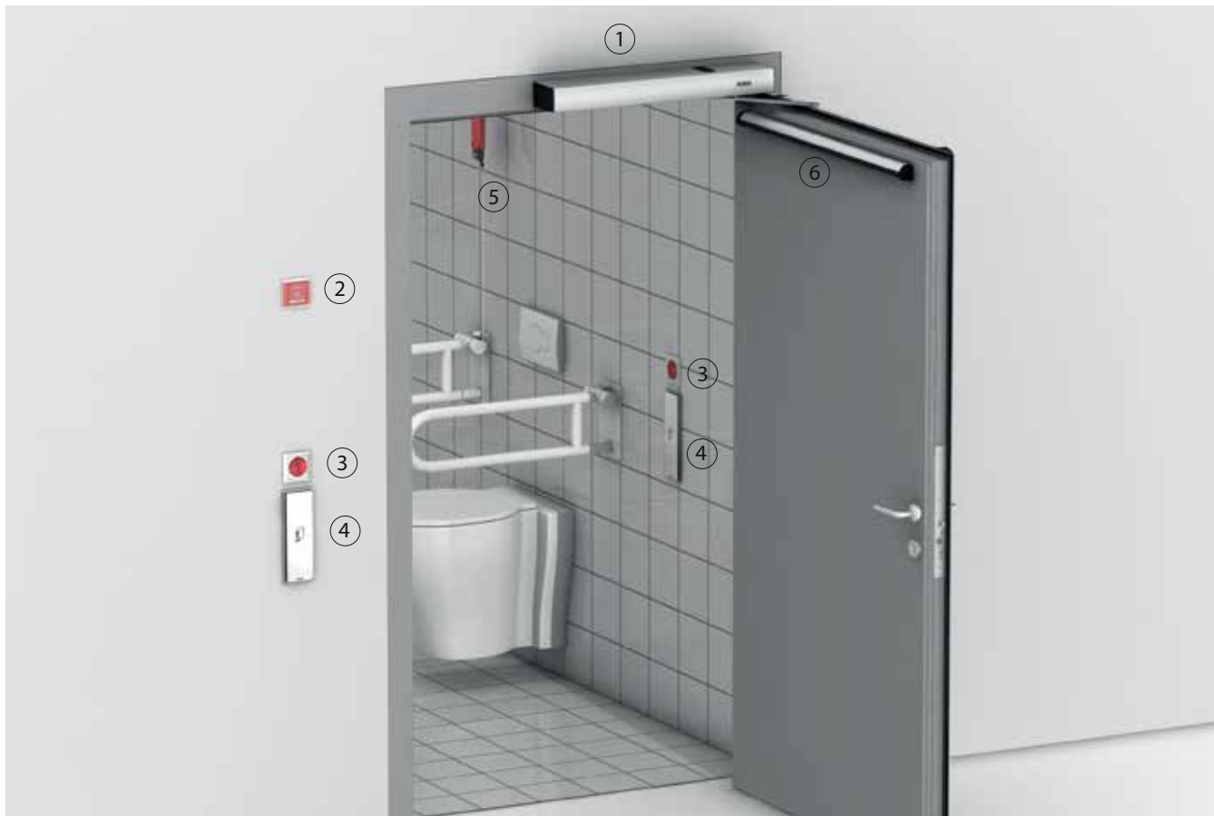
1 = Swing door drive | 2 = Emergency-stop switch (recommended installation height: 1600 mm) | 3 = "Occupied" indicator light | 4 = Elbow switch DOOR OPEN (indoors and outside) | 5 = Pull switch emergency call | 6 = Sensor strip
