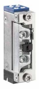
The compact electric strike A5011 is convincing with its small size.. It also has a microswitch (feedback) which is activated by the lock latch. With an unlocking lever the electric strike can be permanently unlocked mechanically.
