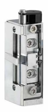
The SILENCE electric strike for fire protection doors FT201SF dampens the swing-back of the strike latch and therefore ensures that it falls back quietly into its starting position. It is perfectly suited for use on fire protection doors in which there should be no swing-back noise due to local conditions.
