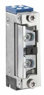
The compact electric strike A5003 is convincing with its small size. It is perfectly suited for use on standard doors and is also approved for use on smoke protection doors. It also has a microswitch (feedback) which is activated by the lock latch.
