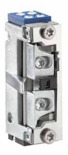
The compact electric strike A5021-F is convincing with its small size. It also has a microswitch (feedback) which is activated by the lock latch. With the 2 mm longer unlocking lever the electric strike can be permanently unlocked mechanically.
