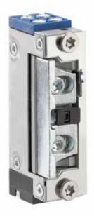
The compact electric strike A5023 is convincing with its small size. It also has a microswitch (feedback) which is activated by the lock latch. With the 2 mm longer unlocking lever the electric strike can be permanently unlocked mechanically.
