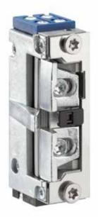
The compact electric strike A5003-F is convincing with its small size. It is perfectly suited for use on standard doors and is also approved for use on smoke protection doors. It also has a microswitch (feedback) which is activated by the lock latch.
