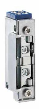
The vector electric strike A4010-K is convincing with its small size and the almost silent opening with direct current even under high preload. With an unlocking lever the electric strike can be permanently unlocked mechanically.
