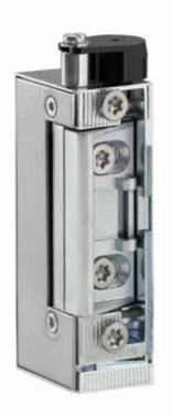
The SILENCE electric strike for fire protection doors FT200S dampens the swing-back of the strike latch and therefore ensures that it falls back quietly into its starting position. It is perfectly suited for use on fire protection doors in which there should be no swing-back noise due to local conditions.
