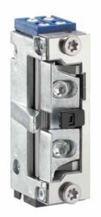
The compact electric strike A5001-F is convincing with its small size. It also has a microswitch (feedback) which is activated by the lock latch.
