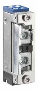
The compact electric strike A5013 is convincing with its small size. It also has a microswitch (feedback) which is activated by the lock latch. With an unlocking lever the electric strike can be permanently unlocked mechanically.
