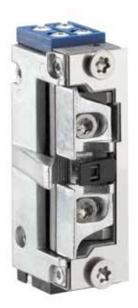
The compact electric strike A5011-F is convincing with its small size. It also has a microswitch (feedback) which is activated by the lock latch. With an unlocking lever the electric strike can be permanently unlocked mechanically.
