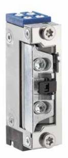
The compact electric strike A5021 is convincing with its small size. It also has a microswitch (feedback) which is activated by the lock latch. With the 2 mm longer unlocking lever the electric strike can be permanently unlocked mechanically.
