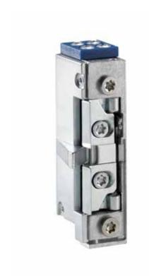
The vector electric strike A4010-F is convincing with its small size and the almost silent opening with direct current even under high preload. With an unlocking lever the electric strike can be permanently unlocked mechanically.
