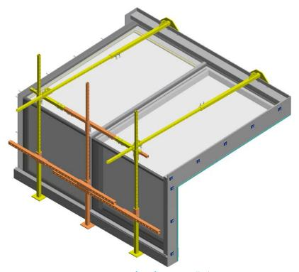
Figure 1 – Lifting frame installed
