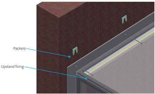
Figure 3 - Wall fixings
