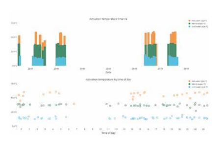
Activation temperature timelines from sensor readings can be easily inspected, to analyse patterns of usage in precise detail.
