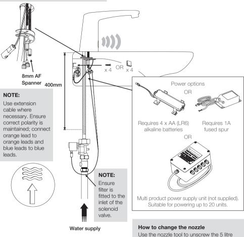
Use the nozzle tool to unscrew the 5 litre (blue) nozzle. Insert the 3.5 litre (blue) nozzle and tighten until flush with tap body; no part should be protruding from the end of the tap. Ensure the nozzle is not over-tightened as this may pinch the "O" ring and cause the tap to leak.
