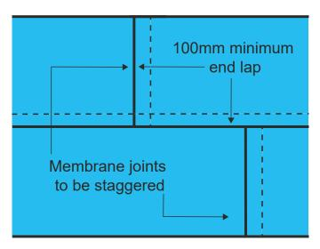
6. End-of-roll overlaps of adjacent lengths should be staggered to avoid them being side by side on adjoining rolls, causing a four fold overlap (See Fig 1).
