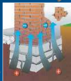
Before system installation - rising damp
