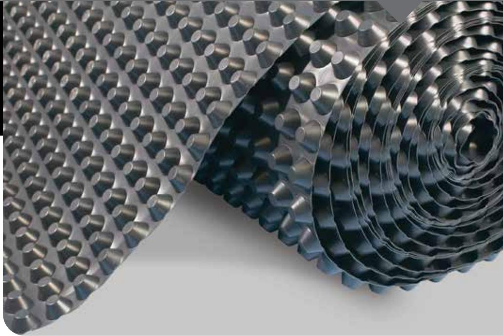
The **CM20 Cavity Drain Membrane** is a 20mm studded membrane, suitable for Type C waterproofing and delivering a grade 3 environment to BS8102:2009 and NHBC Chapter 5.4. CM20 is the highest drainage capacity membrane in the Wykamol Waterproofing range.
