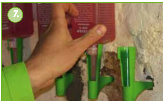
The Capillary Rod must not be prewetted anymore. The nozzles of the cartridges sit directly on the capillary rod providing material to be soaked in.
