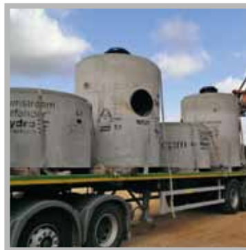
Hydro International Downstream Defenders® with vortex separator
