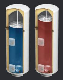
As the water heats up it expands and compresses the air pocket at the top of the cylinder; a floating baffle separates the air from the water.
