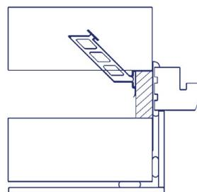
Fig.2 Fully rebated check reveal
