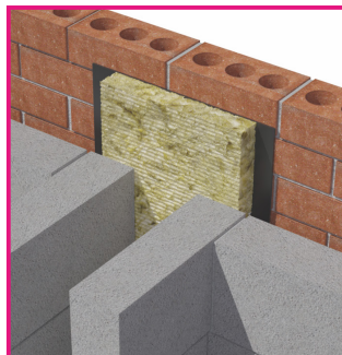
Junction between external cavity wall and party wall
