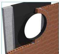
frame construction, the cavity tray flap should be mechanically fixed to the inner leaf
