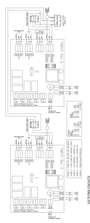
The alarm relays 1 and 2 energize on a fault. The alarm relays 3, 4 & 5 de-energize on a fault, thus activating the low-pressure/high-pressure faults and boiler chiller interlock if the pressurisation unit is isolated from the electrical supply.
