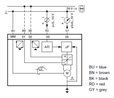
The direction of response to the 0-10V control signal is reversible.
