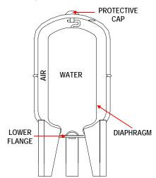
Replacing the diaphragm on the 100, 200, 300, 500 and 750 Litre vessels:
