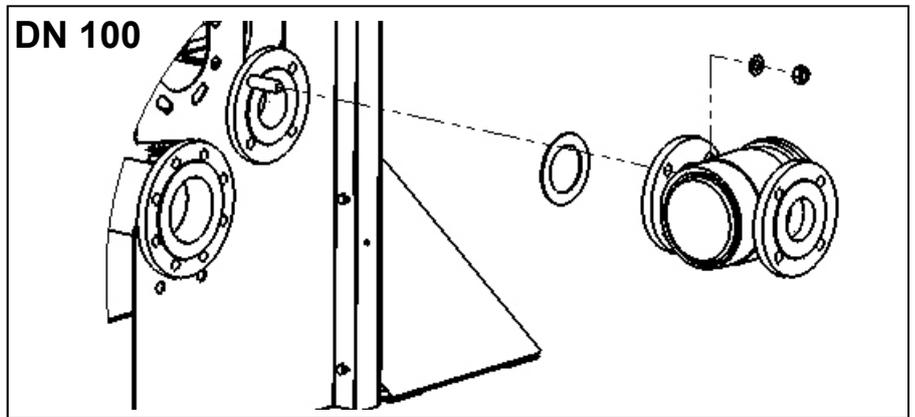
If required by the situation, an extension pipe (optional) can be used to move the location of the gas filter a bit further from the cascade system.
