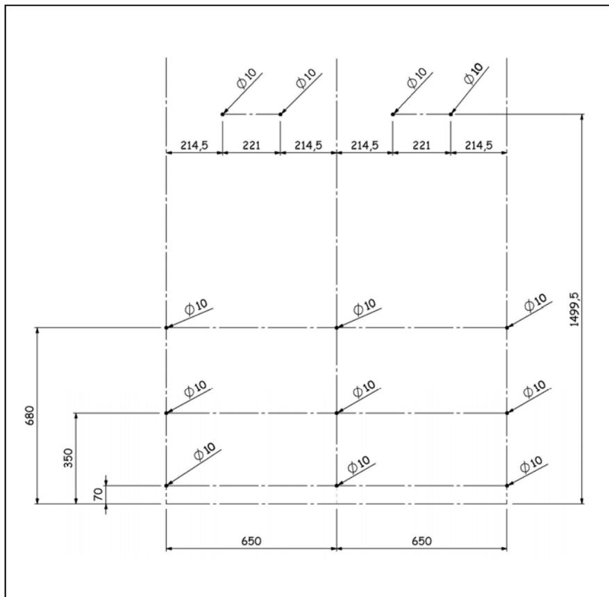
Fix the boiler supports and collector support panels to the wall.
