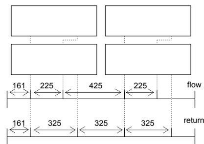
For line configurations of more than 3 boilers and back to back configurations of more than 6 boilers, two collectors have to be connected.
