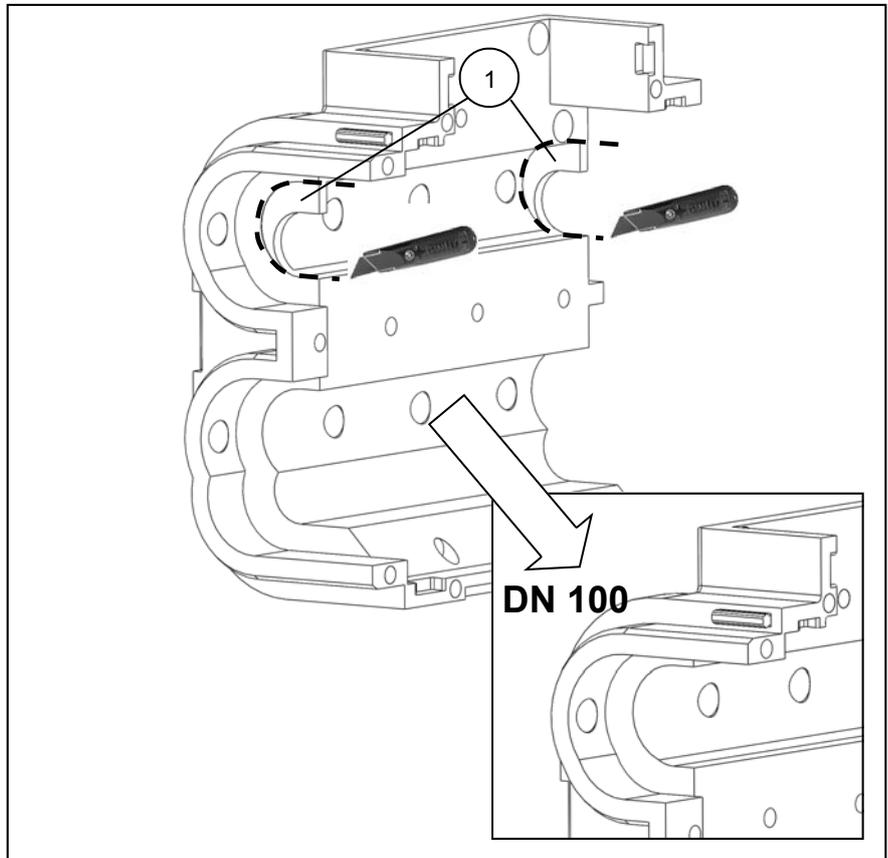
Front panel assembly boiler 1 (left):
