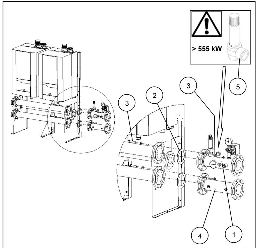
Assemble the ISPESL gas valve to the gas connection as shown in the pictures.
