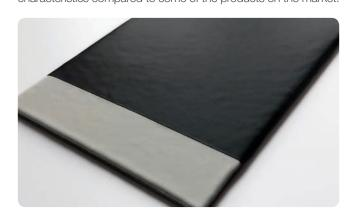
FIRETEX® FX6002 provides a smooth aesthetically pleasing finish for use up to C5 environments when an appropriate top coat is used.
