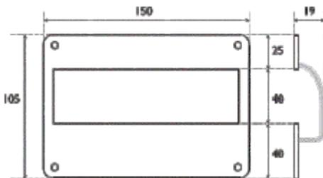
Contact our sales office for advice on back to back fixing of flush pulls. We recommend that these products are installed with intumescent pads
