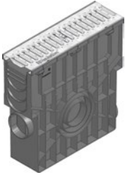
Trash box with PE mud bucket and slotted grating SW 80/10 mm, class A 15, locked
