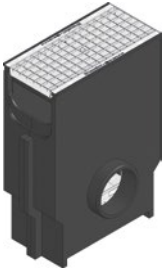
Trash box with mesh grating MW 30/30 mm, galvanised, class B 125, locked
