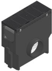
Trash box with galvanised mud bucket and longitudinal ductile iron grating SW 9 mm, KTL, class C 250, locked
