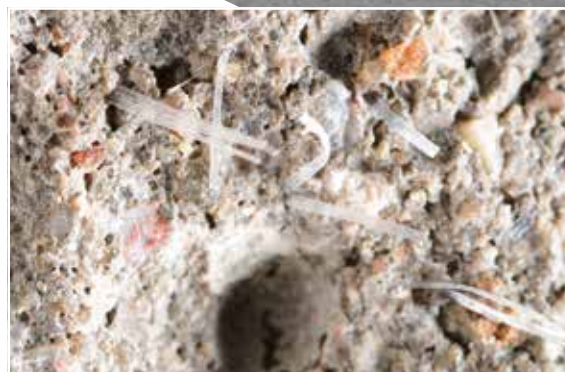
Enlarged view of FASERFIX concrete. The photograph clearly shows the fibres which give the material its great strength.
