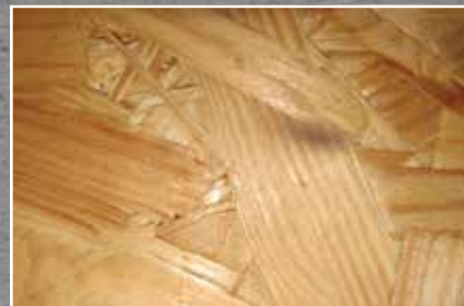
Woodchip board achieves its great strength with the help of a closely interlinked fibre network.
