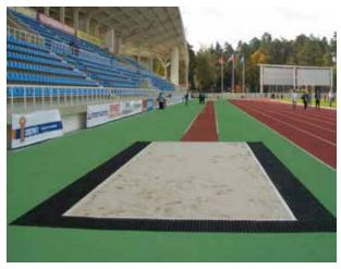
Sand pitch with sand trap channels
