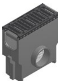
Trash box with galvanised bucket, with ductile iron grating, black, SW 18 mm, class E 600, 4-fold bolted
