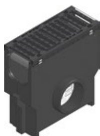
Trash box with galvanised bucket, with ductile iron grating, black, SW 18 mm, class D 400, 4-fold bolted
