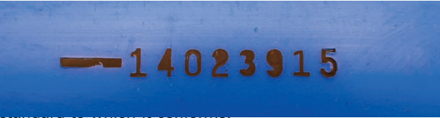
Shift code for a PE100 pipe
