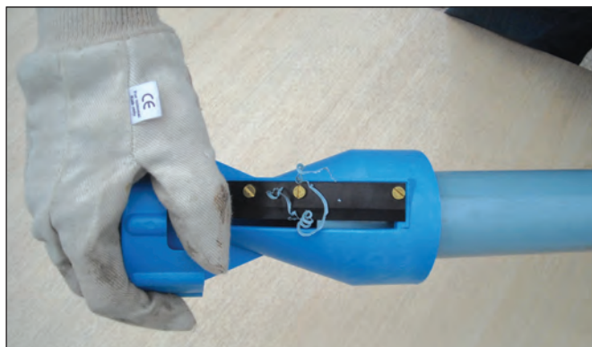
3. Chamfer end of pipe using a chamfering tool or file.
