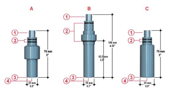
A Submersible PH650, ORP650 B In-line PH660, ORP660 C Insertion/Hot-tap PH655, ORP655 1 BNC receptacle 2 Viton O-rings 3 Porous HDPE junction 4 pH glass or platinum
