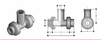
NPT Female Threaded PVC Tee Fittings for ASTM SCH. 80 pipes (NPT threaded female ends)
