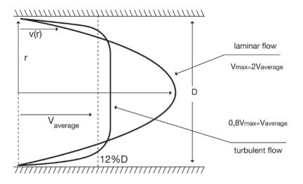
All velocity based flow sensors provide an accurate and reliable indication only when they are measuring a fully developed turbulent flow. Fully developed turbulent flow occurs in every Newtonian fluid when the Reynolds Number is greater than 4500.
