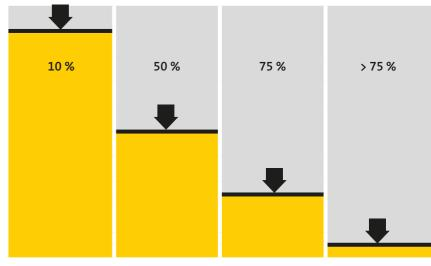
At 10 % compression - Soundproofing and anti-vibration
