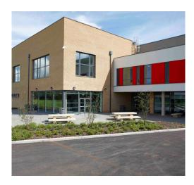
At the £16m Yate International Academy 215 windows were installed in the Passivhaus certified GENEO® window system. These are WER A rated with a Uw-Value of just  $1.2 \text{W/m}^2 \text{K}$ . This was in line with the overall specification of the Academy which focuses on sustainable features including a ground source heat pump powered by photovoltaic panels and highly insulated materials throughout.
