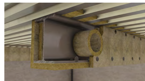
Figure 9 Beam with circular holes (boxed protection - dry joints)
