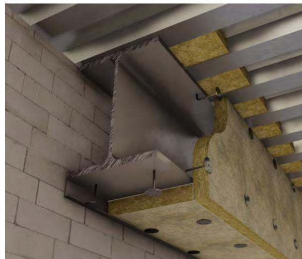
Figure 3 Two-sided protection with stud welded pins (Up to 3 hours fire protection)
