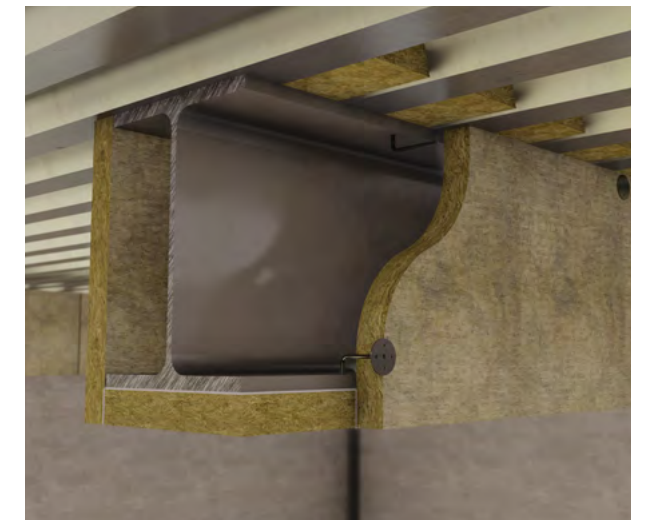
Figure 5 Stud welded pins and board-to-board glued joints (Up to 4 hours fire protection)
