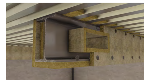
Figure 10 Beam with square or rectangular holes (boxed protection - dry joints)
