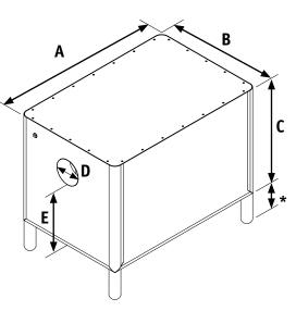
Above ground separator has a smooth cover plate and is supplied with height adjustable feet which increase dimension 'C' by 100 - 125mm.
