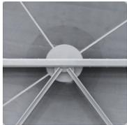
FläktGroups RegAsorp is a hygroscopic rotor with a proprietary zeolite surface treatment of 4 Å (angstrom). This rotor is more efficient than traditional types in absorbing moisture. The molecular grid of 4Å permits water vapour to be transferred while pollutants, which typically have larger molecules, are not carried over.
