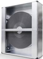
Rotary heat exchangers are used for heating and cooling recovery in air handling systems and typically enhances their efficiency. The rotary heat exchangers main component is the rotor, which is made of either thin folded sheet aluminium or micro-glass, formed as triangular pipes.
