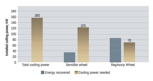
The installed cooling capacity is reduced from 160 kW to 70 kW and the energy consumption is reduced by 1700 kWh. This brings a significant reduction in the size of the chiller and cooling energy savings.
