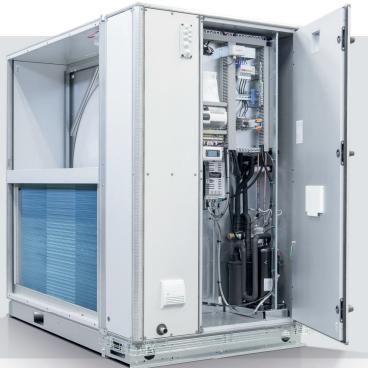
Our ReCooler HP offers an air handling unit with an integrated DX cooling system. There is no need to mount cooling equipment on the roof of the building and installation is quick and simple as the ReCooler HP is factory tested and ready to run after local inspection requirements have been fulfilled.
