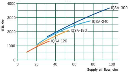
The diagram shows the approximate cooling effect  $P_{tot}$  in BTU/hr with water flow  $q_w$  = 0.8 GPM, temperature difference between room air and supply air  $\Delta t$  = 14°F, difference between room air and average water temperature = 14°F, pressure drop 0.25 in w.g. on the air side and maximum sound pressure level  $L_{a10}$  = 34 dB(A).
