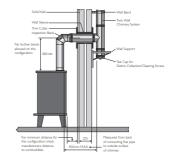
NB Where the connecting flue pipe from the appliance passes through any wall other than the existing chimney wall, the connecting flue pipe must be a System Chimney of twin wall insulated design.
