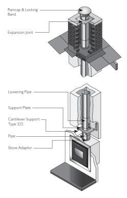
CONNECTING FLUE PIPE ON CONDENSING BOILER
