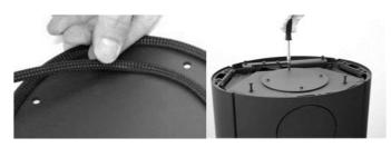
2.) Stick the cover for the upper flue pipe (accessory part #1) with the seal for the central supply air feed (accessory part #3) above and below the screw holes and attach to the stove.
