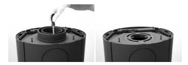
1.) Remove the top plate and take off the outer air inlet and inner flue tube supports
