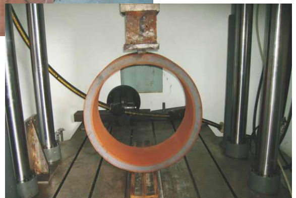
Opposite: Pipe being type tested in accordance with EN295-7 Clause 4.3.1. Strength
