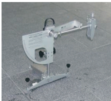
Pendulum Test Machine (image courtesy of HSE)
