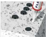
Discs should sit between 0.5mm and 1.00mm proud of the step surface when installed and therefore a preformed hole should be created which is of adequate diameter and depth to accept the disc and sufficient adhesive to affix it.
