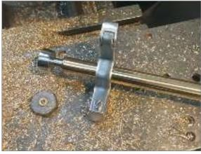
C.A.T. stair rods and eyes are made from solid brass. Stair rods are made to customer order from sizes supplied and are hand lathe turned prior to polishing and finishing.
