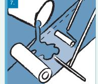
Ensure all air pockets are removed during the installation by rolling towards the edges of the fleece.
