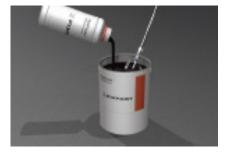
Pour contents of PPR-5000 (Part B) bottle into PPR-5000 (Part A) tin. Thoroughly mix the two components for 3-5 mins using PPR-WHISK with a power drill.
