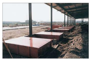
Levellers in heavy-duty fabricated steel pouring pans
