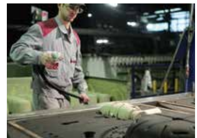
Insertion of the sand core
