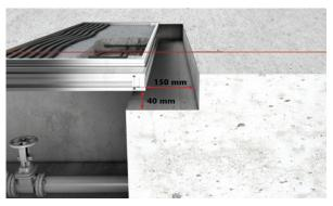
**Step 2:** A minimum rebate of 150mm wider than the over frame size and 40mm deeper than the over frame height of the access cover is to be provided for bedding and haunch material.
