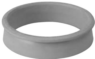
The GM-X-VACplus sealing element allows the vacuum installations with „standard socket Type A1“. The seal is manufactured from EPDM and is provided with two flexible lip sealing elements. The outer lip
