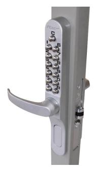
The narrow stile Keylex 700AR design, with its built-in clutch mechanism protecting the lock furniture, will suit stile widths down to 45mm in this configuration and is particularly suited for use on aluminium and hollow metal door sections. The Keylex 700AR can be expected to give many years' service if specified and maintained correctly.
